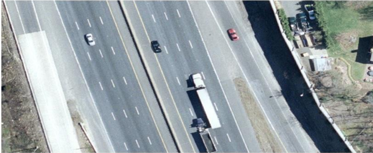
outside right-of-way shoulder on roadway gore shoulder on roadway separator shoulder on roadway shoulder gore on roadway shoulder roadside outside right-of-way
